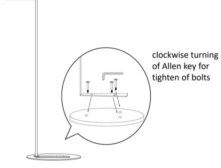
STEP 6: Use Allen key to fix the bracket to timber block at bottom of sofa with three bolts M6X50.
