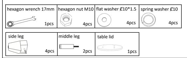
STEP 2: Make the screw of side leg go into hole at corner of bottom frame, then place flat washer, spring washer and hexagon nut on the screw in turn, finally use hexagon wrench to fasten hexagon nut tightly.
